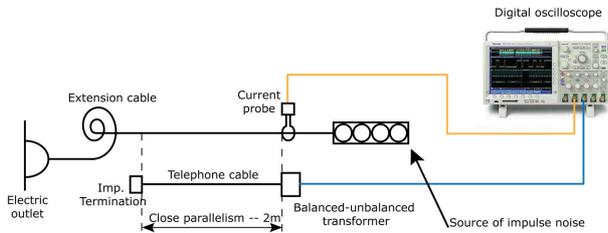
Figure 1. Setup of a workplace for impulse noise diagnostics.
