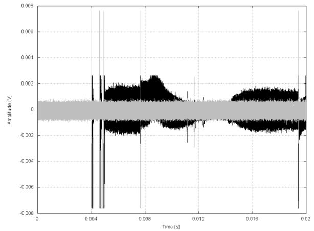
Figure 9. Startup of a drill.
