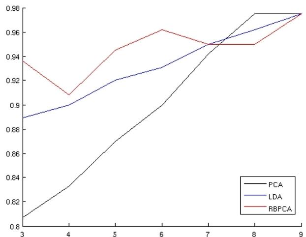
Figure 5. Comparison between correct classification rates for PCA/LDA+NN and the proposed *RBPCA MaxLike* classifier in ORL
