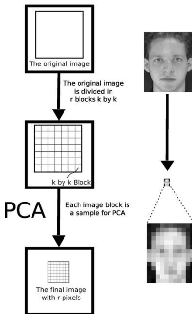
Figure 1. Illustrative diagram of the proposed Block-Based PCA.
