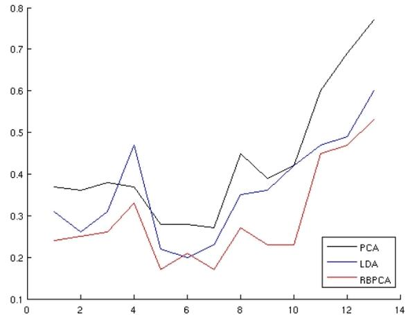
Figure 8. Classification errors for each possible variation using PCA/LDA+NN and the proposed *RBPCA MaxLike* method using 88-D feature vectors.
