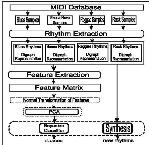
Figure 2. Block diagram of the proposed methodology.
